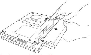
Sample removing the discharged battery
